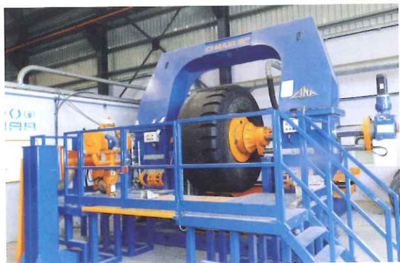
Cima Impianti offers a range of equipment that includes CNC peeling, buffing and grooving machines (pictured) along with a line of CNC extruders, skive fillers and cushion gum application machines Cima Impianti bietet CNC-gesteuerte Schäl- und Raumaschinen genauso an wie solche, um Profile in Slickreifen zu schneiden (Smooth & Groove)
